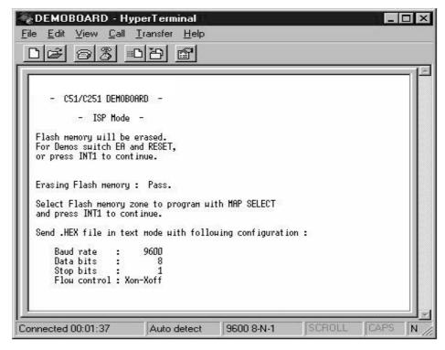
Turn on the C51/C251 Demo Board and then follow the instructions on the terminal screen and LCD display. After erasing Flash, the program asks for the memory zone, and then asks to send the HEX file in text mode (see Figure 3-4, Figure 3-5 & Figure 3-6).
